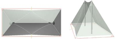
5. Now pull out each strut supported corner and stake. Line tighteners adjust tension. Pull cord end to tighten, lift lever to loosen. Lower tightener tensions perimeter, upper tightener tensions upper panels.
