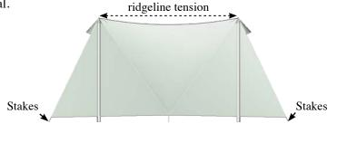
4. Restake corners as necessary so that the canopy corners form a rectangle and the ridgeline is taut.
