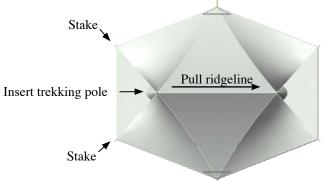
3. Pull canopy ridgeline out. Insert second pole through other vent into grommet. Stake opposite door so that door corners are taut and poles are vertical.
