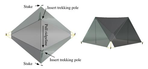
3. Now insert end pole tip into grommet or, if using talller trekking pole, into O-ring. While holding top of pole, remove end cording from initial stake and tension off to side as shown.
