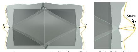
goes into grommet on underside of vent. Stake vestibule. Pull ridgeline across and repeat on other side so that the structure looks like this:
