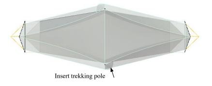
6. Set pole vertically and pull canopy ridgeline out. Be sure vestibule ends are hooked together. Stake cording at end of vestibule.
