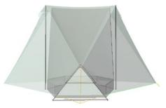
8. Use line tighteners (pull cord end to tighten; lift lever to loosen) to adjust tension. Tighten ridgeline first, then tighten perimeter. Adjust end tensions and vertical pole positions until shape is symmetrical and ridgeline is only slightly curved.
